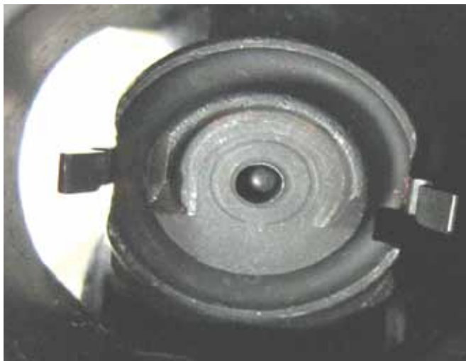
Figure 2: XREP "Old Version" showing protruding ring around edge of breechface
